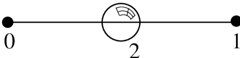
Fig. 10: P_1 Lagrange element on a segment with additional internal bubble function, 3 d.o.f., C^0
