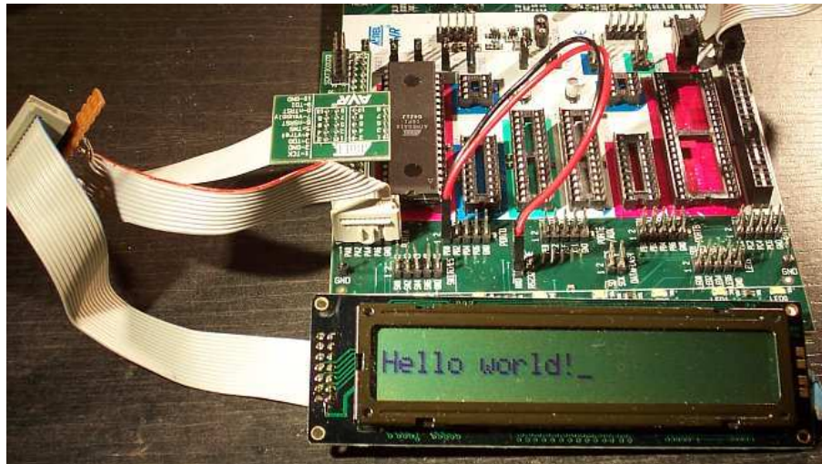
Figure 9: Wiring of the STK500
