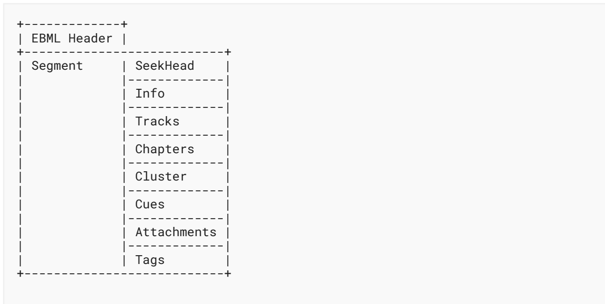
Figure 1: Basic Layout of a Matroska File
