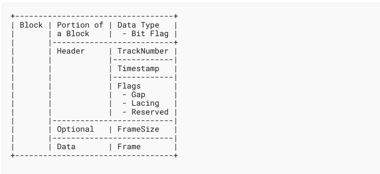
Figure 7: Representation of the Block Element Structure
