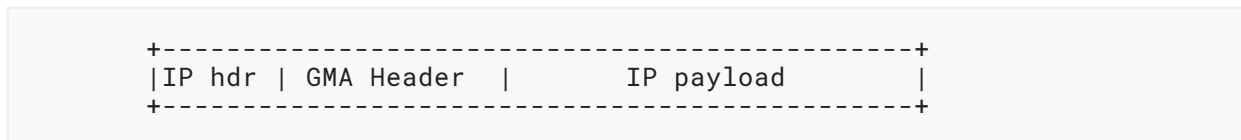
Figure 5: GMA PDU Format with Header-Based IP Encapsulation
