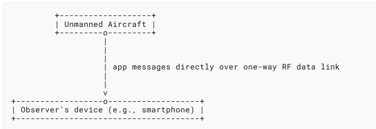
Figure 4: Broadcast RID Information Flow
