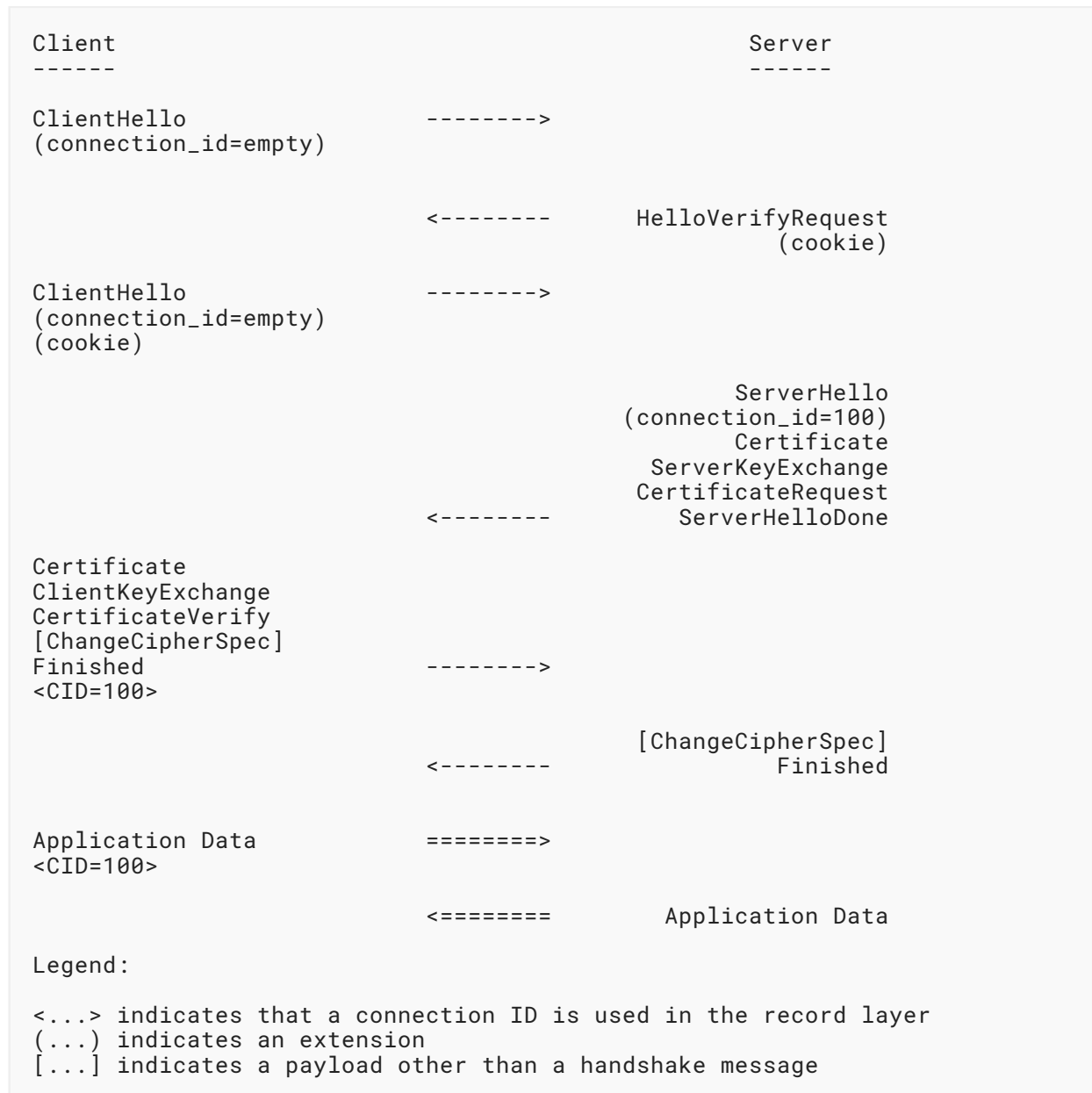
Figure 4: Example DTLS 1.2 Exchange with CID
