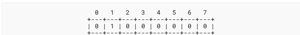
Figure 19: Dispatch Format for Uncompressed CCNx Interest Messages
