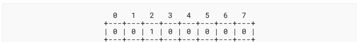
Figure 15: Dispatch Format for Uncompressed NDN Data Messages
