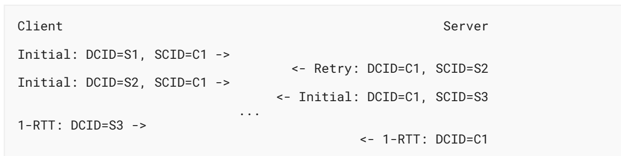
Figure 8: Use of Connection IDs in a Handshake with Retry
