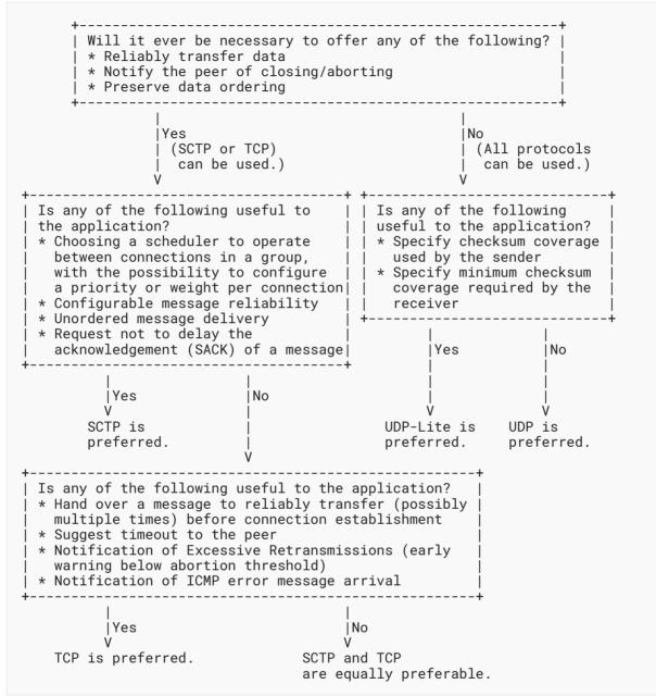
Note that this decision tree is not optimal for all cases. For example, if an application wants to use "Specify checksum coverage used by the sender", which is only offered by UDP-Lite, and "Configure priority or weight for a scheduler", which is only offered by SCTP, the above decision tree will always choose UDP-Lite, making it impossible to use SCTP's schedulers with priorities between grouped connections. Also, several other factors may influence the decisions for or
