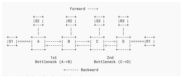
Figure 7: Testbed Topology for Multiple Bottlenecks
