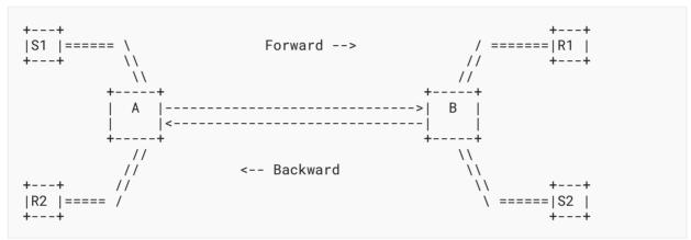
Figure 4: Testbed Topology for Congested Feedback Link
