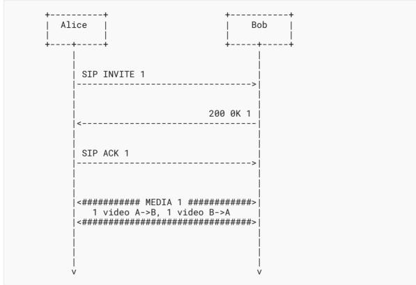
In SIP INVITE 1, Alice sends Bob a SIP INVITE including the basic audio and video capabilities and data channel in the SDP body as per [RFC8841]. Alice also includes the "sip.clue" media feature tag in the INVITE. A snippet of the SDP showing the grouping attribute and the video
